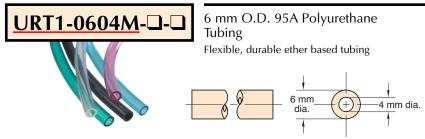
Working Range: 0 to 105 psig at 100°F Maximum 120°F Static Burst Pressure: Over 450 psig at 70°F
