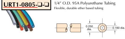
Working Range: 0 to 105 psig at 100°F Maximum 120°F Static Burst Pressure: Over 450 psig at 70°F
