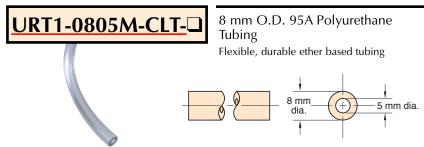
Working Range: 0 to 105 psig at 100°F Maximum 120°F Static Burst Pressure: Over 465 psig at 75°F
